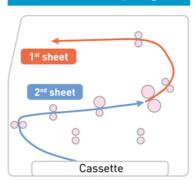
After printing both sides of 1<sup>st</sup> sheet, printing of 2<sup>nd</sup> sheet starts.
