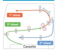
After printing the back of 1<sup>st</sup> sheet, printing the back of 2<sup>nd</sup> sheet starts. After printing the front of 1<sup>st</sup> sheet, printing the back of 3<sup>rd</sup> sheet starts.
