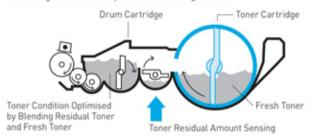
The lifetime of the drum cartridge depends on the effects of stress applied to the toner inside the cartridge. In order to increase the lifetime of the cartridge with a reduction in toner stress, Panasonic's new drum cartridge controls the amount of toner supplied to the drum cartridge by sensing the toner residual amount and optimises the proportion of fresh & residual toner in the drum cartridge.
