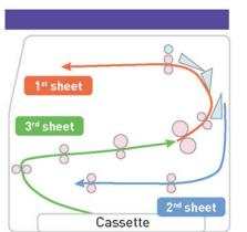
After printing the back of 1st sheet, printing the back of 2<sup>nd</sup> sheet starts. After printing the front of 1st sheet, printing the back of 3rd sheet starts.
