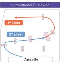
After printing both sides of 1st sheet, printing of 2<sup>nd</sup> sheet starts.
